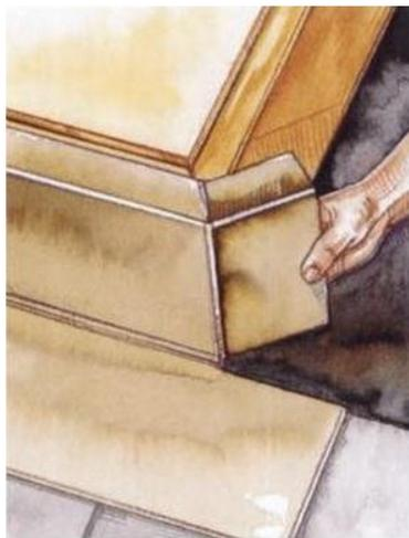
Cut the horizontal flanges of the bottom piece of skylight flashing and wrap the ends around the frame sides.
