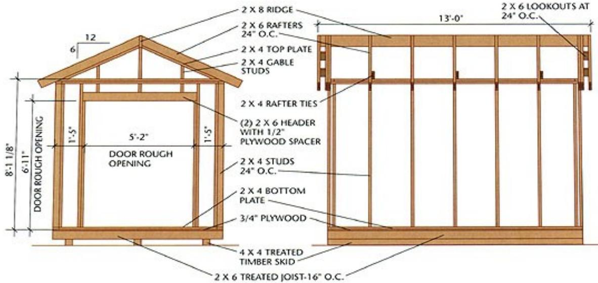
FRONT FRAMING ELEVATION
