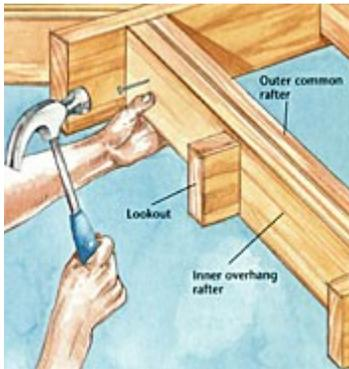
Attach lookouts to four of the overhang rafters, then nail the overhang rafters to the outer common rafters.
