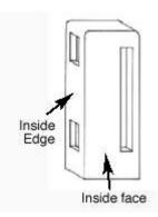
**1.** On the inside (3/4") edge, make a rout that is 1/4" deep and 1/2" wide that runs from 1/2" from the top of the leg to 2 1/2" from the top. This rout should be 1/8" in from each side. This slot will accommodate the top support that runs along the length of the rack.
